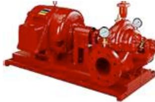
Fire pumps are needed whenever pressure requirements of a fire protection system exceed the capabilities of the available water supply. Two types of pumps are typically used: centrifugal fire pumps, where water is available to supply the pump under pressure, such as a city supply; and vertical turbine pumps, where the available water supply is in a static state, such as a pond or reservoir.
