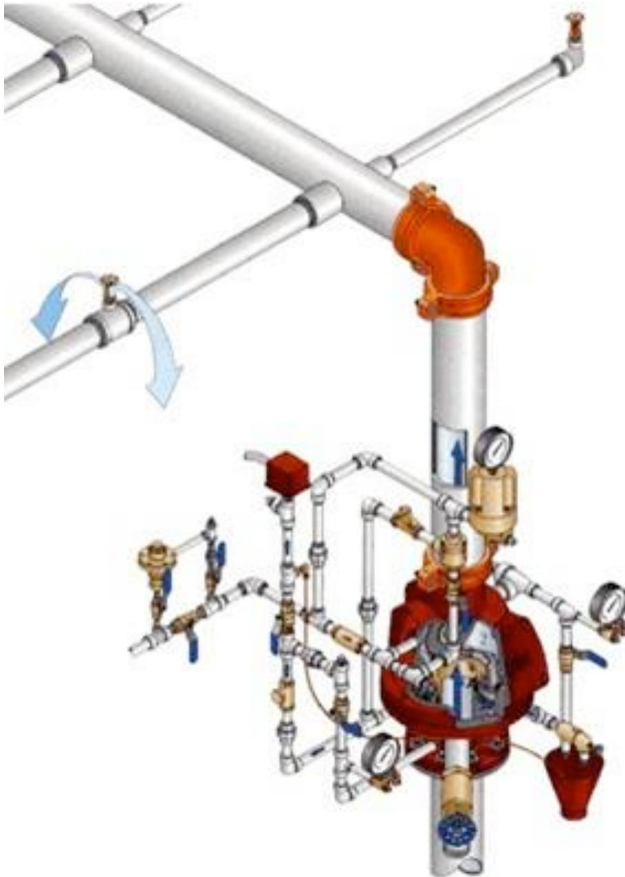
**Preaction and Deluge** – Preaction systems and deluge systems required fire detectors (smoke, heat, etc.) for the actuation of the system. A deluge system uses open sprinklers or nozzles, so that all flow water is discharged when the deluge valve actuates. Deluge systems can be used for occupancies where the hazard is considered severe, such as with flammable liquid hazards where the fire could spread over a large floor area.
