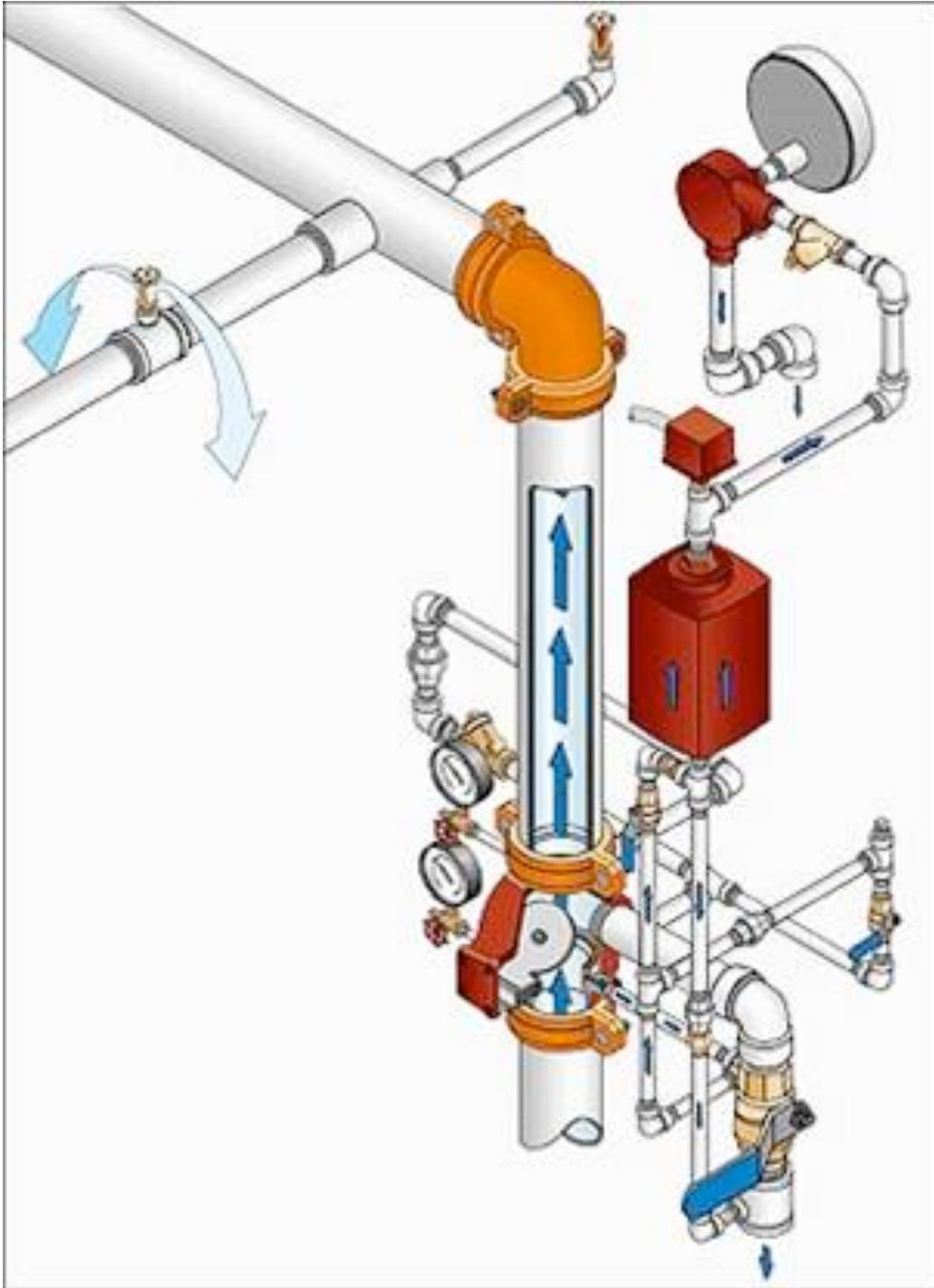
**Dry** – In areas where low temperatures could cause a wet pipe system to freeze, a dry pipe system is intended for use. Dry pipe systems are pressurized with air in the ambient condition and experience an inherent delay in the discharge of water to
